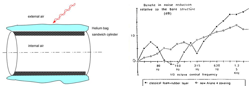
Figure 6. Helium bag to reducing noise inside fairing.
