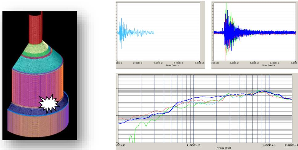
Figure 14. SEA-Shock prediction of Ariane 5 separation test of the upper part (top synthesized and measured time history on the payload, bottom SRS for predicted time signal (blue) compared to SRS from measurements).
