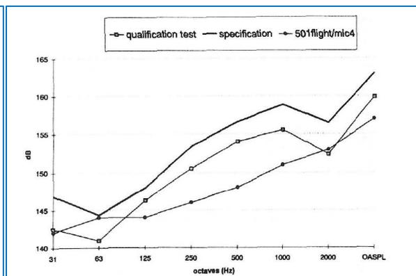
Figure 13. Comparing qualification test and flight 501 measurement.
