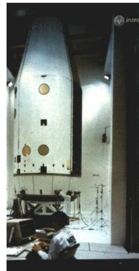
Figure 3. Combined BEM/SEA prediction (left) of the noise reduction of Ariane 4 fairing tested in reverberant chamber (right).
