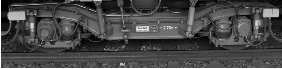
Figure 1. Bogie featuring primary rubber elements [6].
