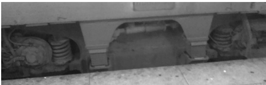
Figure 1. Motor bogie on SNCF BB 22200, 2 ary suspension with stacked metal/rubber layers.
