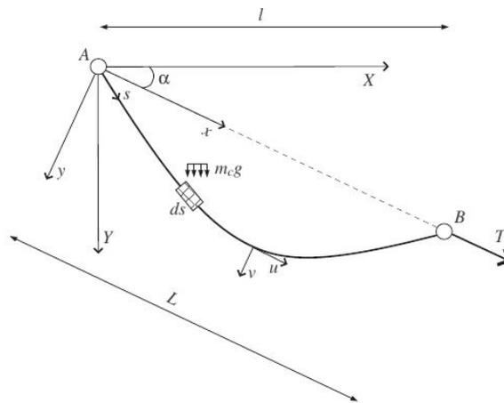
Figure 1. Static equilibrium configuration of a suspended cable
