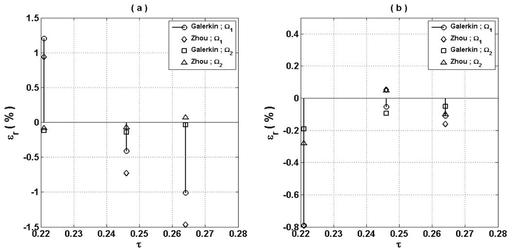
Figure 2: Relative errors  $\epsilon_r(\%)$  related to the 1<sup>st</sup> and 2<sup>nd</sup> dimensionless frequencies  $\Omega_{1,2}$  with respect to results obtained by both Galerkin and Zhou's methods and presented in [3] for inclined cables with: (a)  $\alpha = 10^\circ$ ; (b)  $\alpha = 60^\circ$ .
